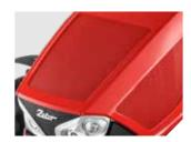
2. The new bonnet design brings better heat dissipation from the tractor's engine compartment.
