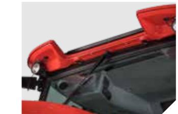
4. The new indented shape of the roof gives a better view from the cabin (for instance, when working with a front loader). Use of new technologies ensures better heat resistance and UV stability.
