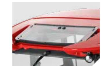
7. The newly shaped sunroof ensures adequate ventilation of the cabin and guarantees a good view of the front loader. The window is equipped with a sun visor and fulfills FOPS protection requirements.
