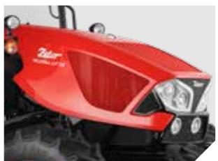
1. The new look is down to new plastics technology, which provides greater heat resistance and UV stability.
