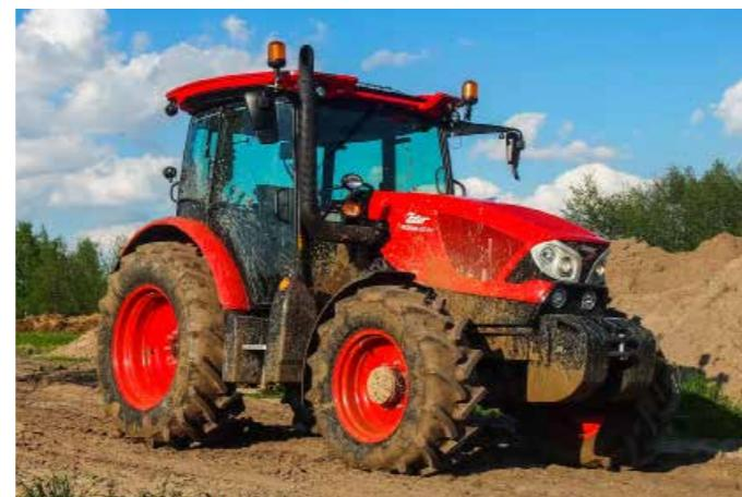
*„The highest power in drag, 57 kW (78 HP), was measured at the speed of 7.8 kph. The loss of power as opposed to the power measured on PTO reached 17 %, which is a normal value for mechanical gearboxes. The connection of 4WD is electric.“*
