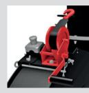
Extra safety and improved ergonomy for lowering discharge pipe with a winch as a standard.
