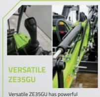
performance and features, which can easily meet customer needs. A high configuration model is equipped with a breaker plumbing, a quick coupler plumbing, and multiple attachment plumbings, and allows the user to control the plumbing with a switch on the joystick for easier operation.
