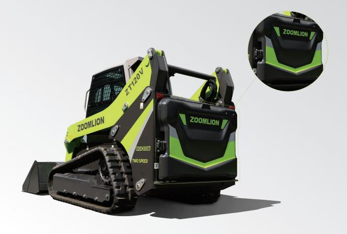
The tailgate is made of 6mm high-strength steel plate, which can resist splashing stones and metal collisions, protecting the engine and pipelines.
