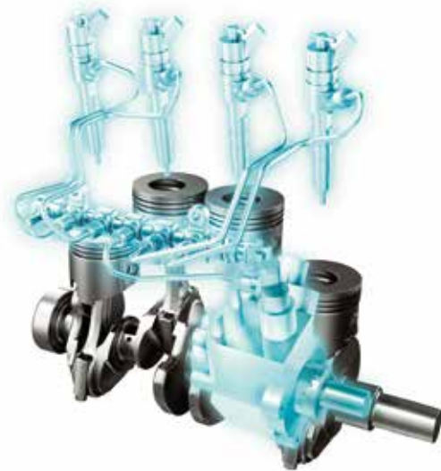
Common-rail Injection system
