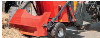
Loading bucket is an **optional** feature that helps operators to load ingredients without external loaders.
