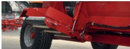
Lateral conveyors allow operators to adjust unloading height. This is a standard feature for horizontal, **optional** for vertical mixer feeders.
