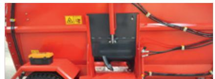
This is an **optional** feature for double auger horizontal mixer feeders that allows operators to unload the feed from both sides of the machine.
