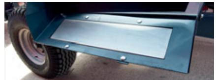
Magnet is an **optional** feature that can be assembled on the discharge point. That feature helps in cleaning the foreign particles from the feed.
